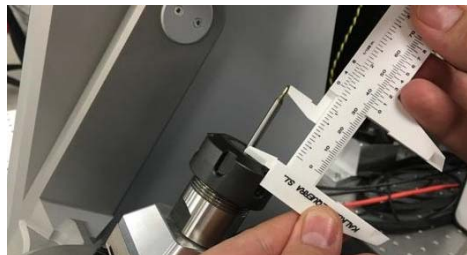
Figure 8.1 Image showing how to measure the length of the sample
