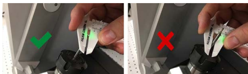
Figure 8.2 Image showing how to measure the diameter of the sample correctly and incorrectly
