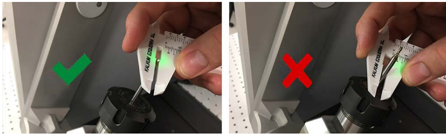
Figure 8.14 Image showing how to measure the diameter of the sample correctly and incorrectly
