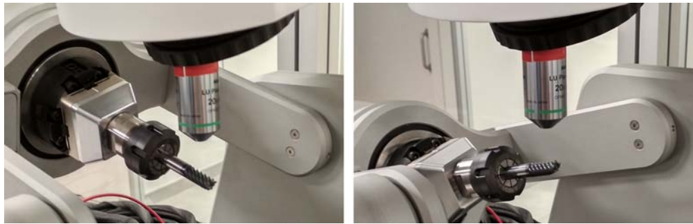
Figure 6.9 Example of the two elevations (-15° and 15°) used in dual mode to measure a milling tool
