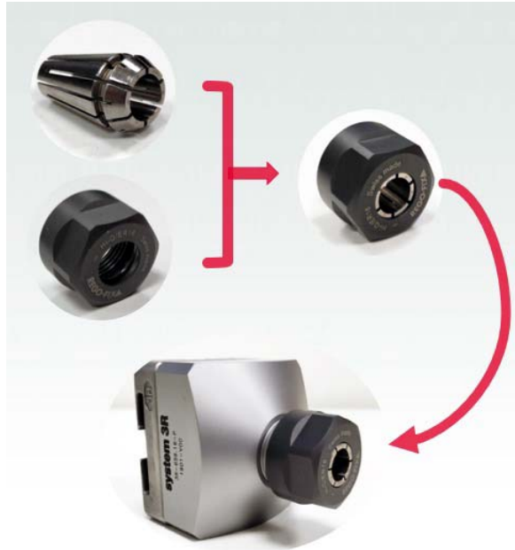
Figure 2.7 Steps to mount the different parts comprised in the collet holder
