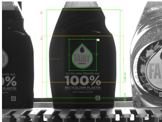
Fig. 234: Case 1: Label correctly applied
