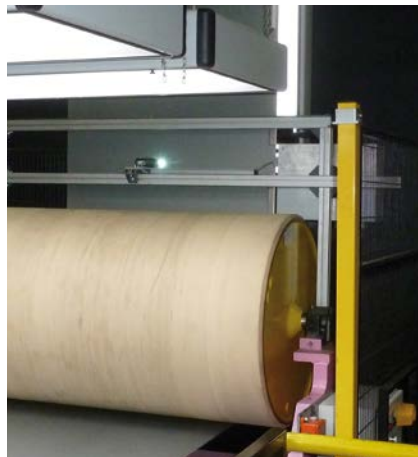
Measurement of the zinc strip color in production
