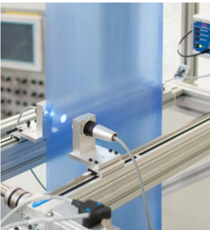
Inline measurement of the color gradient of glass, Plexiglas®, PET and PVC films and paper
