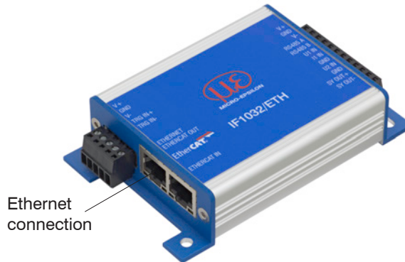
Fig. 5 Ethernet connection for a LAN or Crossover cable
