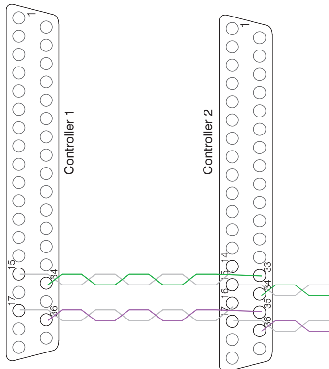
Fig. 31 Synchronization wiring for two controllers
