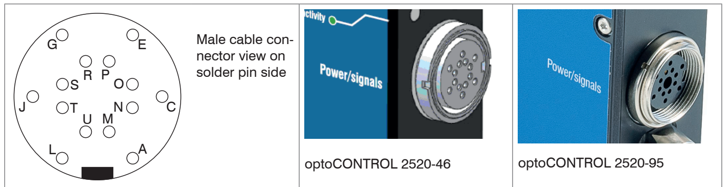
Fig. 27 14-pin. male cable connector for supply and signals
