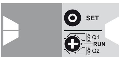
ILR103x: Adjust analog output and switching output via touch keys
